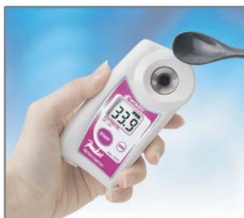
① Place the sample onto the prism surface.
