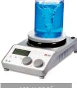
MS-H-PRO φ135mm(5 inch) stainless steel cover with ceramic Brushless DC motor 18W 10W 550W 500W 100~120/200~240V 50/60Hz 20L 80mm 100~1500rpm resolution±1rpm LCD LCD Room temp.-340°C increment 1°C ±1°C(<100°C) ±1%(>100°C) 360°C ±0.1°C PT1000 (accuracy ±0.2) 50°C 1min to 99h 59min RS232 IP42 160×280×85mm
