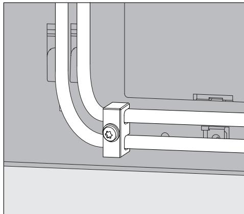
The strain relief provided with the dispensing modules for the dispensing hoses is fitted to the bottom right-hand side of the back of the machine to prevent the hoses from dislodging themselves from the dispenser connections during use.
