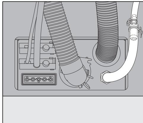
The hose adapter for dispenser connections with larger diameters is supplied with the DOS G 80 and must be used with G 8066 and PG 8067 commercial dishwashers.
