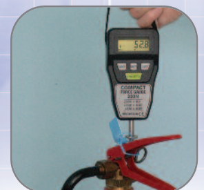
Testing fire extinguisher
