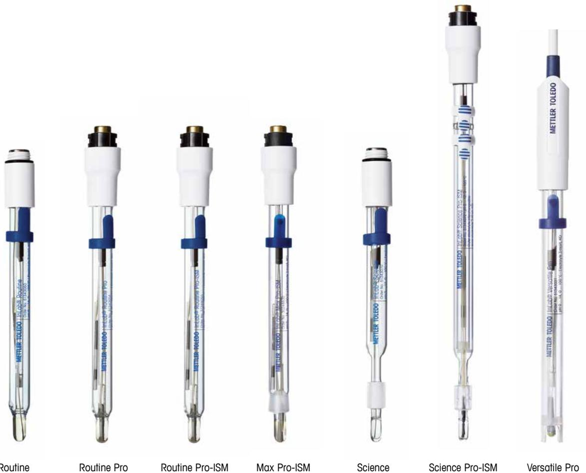
Electroplating is a common technique used to coat metals in order to add desired properties to them. Strong acids and bases are needed for this process and the robust HA glass of the InLab Routine Pro-ISM is ideal for this application as it covers the whole pH range with an extremely low alkali error.
