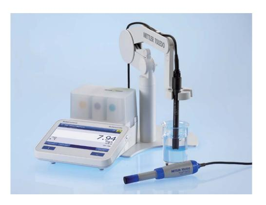
The SevenExcellence S900 benchtop instrument provides customers a premium benchtop solution to measure dissolved oxygen (DO) in aqueous media. Whether you measure DO using the traditional polarographic or the new digital optical dissolved oxygen technology (OptiOx), the S900 guarantees precise and highly reproducible results.
