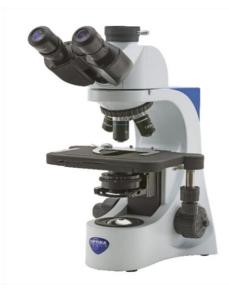
Trinocular brightfield microscope, 1000x, IOS N-PLAN objectives
