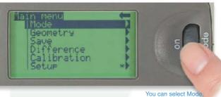
A wide array of display modes (corresponding to six languages) Geometry selection Difference, and Calibration from the Main Menu screen.
