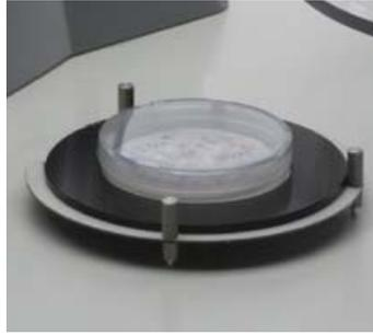
For central positioning of Petri dishes up to Ø 60 mm.
