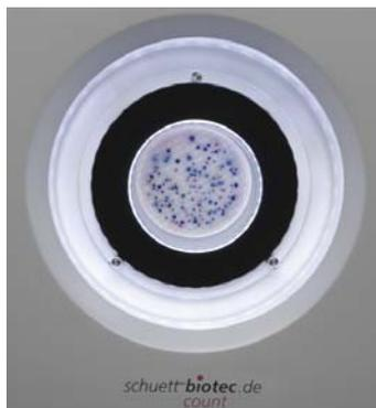
Various coloured colonies on filter disk with adapter for Petri dishes with  $\varnothing$  50-60 mm.
